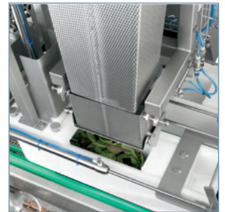
An example of a custom-built Bilwinco distribution tool for pre-cut lettuce leaves. The internal surface of the tool is optimised for lettuce.
